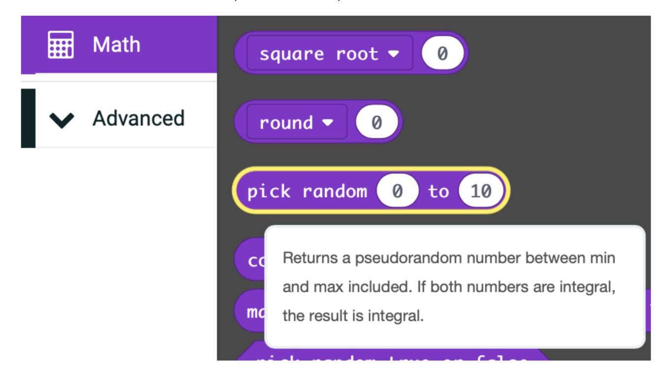
Drag the "pick random" block onto the workspace and join to the "set random" block. A random number between 0 and 1 will give us the 2 options needed.
