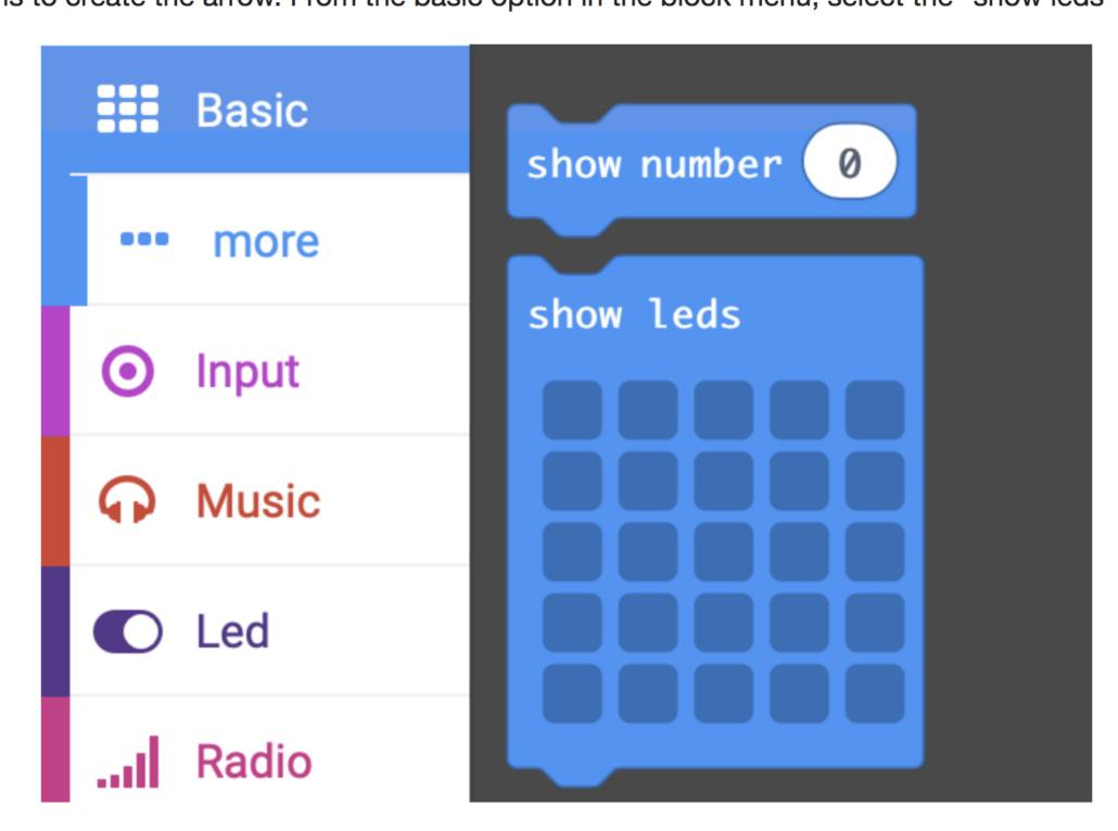
Drag the "Show leds" block onto the workspace and draw the pattern by clicking on the boxes that you want to light up. A white square indicates LED on.
