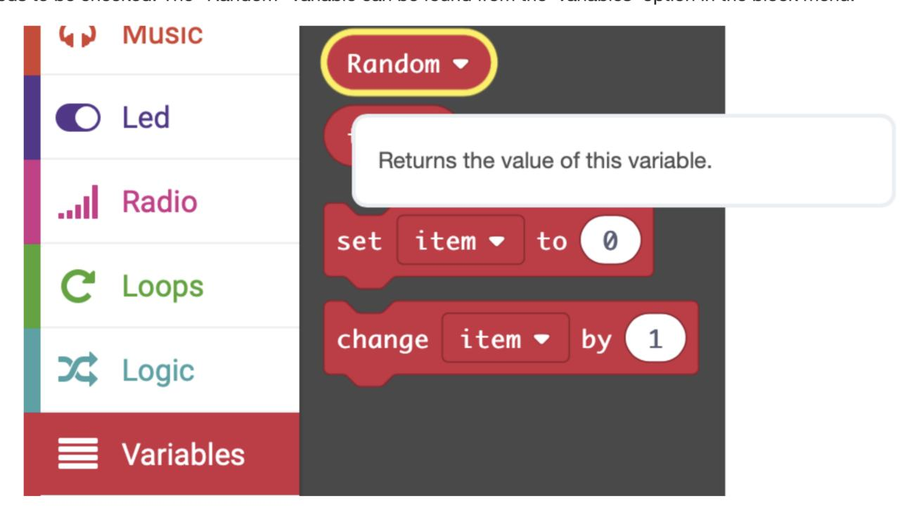
The "Random" variable block is placed in the "equals" block to test the IF statement logic. If the "Random" variable contains a "0" the first option is selected otherwise the second option is chosen.
